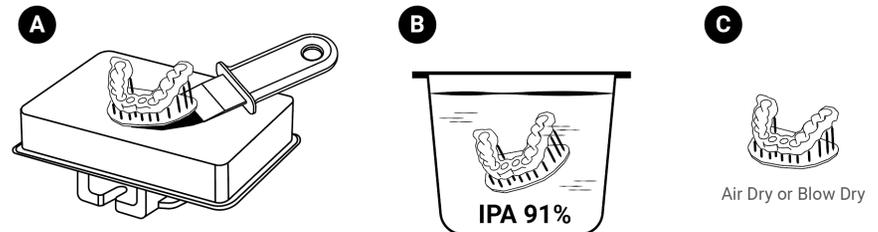
In total, the print should spend no more than **10 minutes** in alcohol to avoid micro-cracks and abrasions. Once cleaned, air-dry the print using compressed air. If the model feels tacky to the touch or has a shine, dunk it in IPA a few more times until the excess resin is totally removed.
