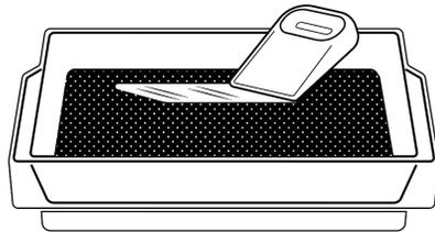
Always stir to homogenize the resin before initiating a new print. Failure to mix resin, especially when topping-off from a bottle, may result in failed prints. Always clean the tank between uses, especially when switching between material types.
