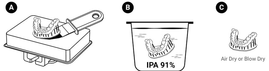
In total, the print should spend no more than **10 minutes** in alcohol to avoid micro-cracks and abrasions. Once cleaned, air-dry the print using compressed air. If the model feels tacky to the touch or has a shine, dunk it in IPA a few more times until the excess resin is totally removed.
