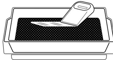
Always stir to homogenize the resin before initiating a new print. Failure to mix resin, especially when topping-off from a bottle, may result in failed prints. Always clean the tank between uses, especially when switching between material types.
