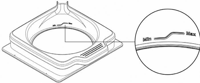
If there is leftover resin in the tank from the previous print, use the provided resin wiper to stir the resin before printing. This ensures that the resin is properly mixed and clean.
